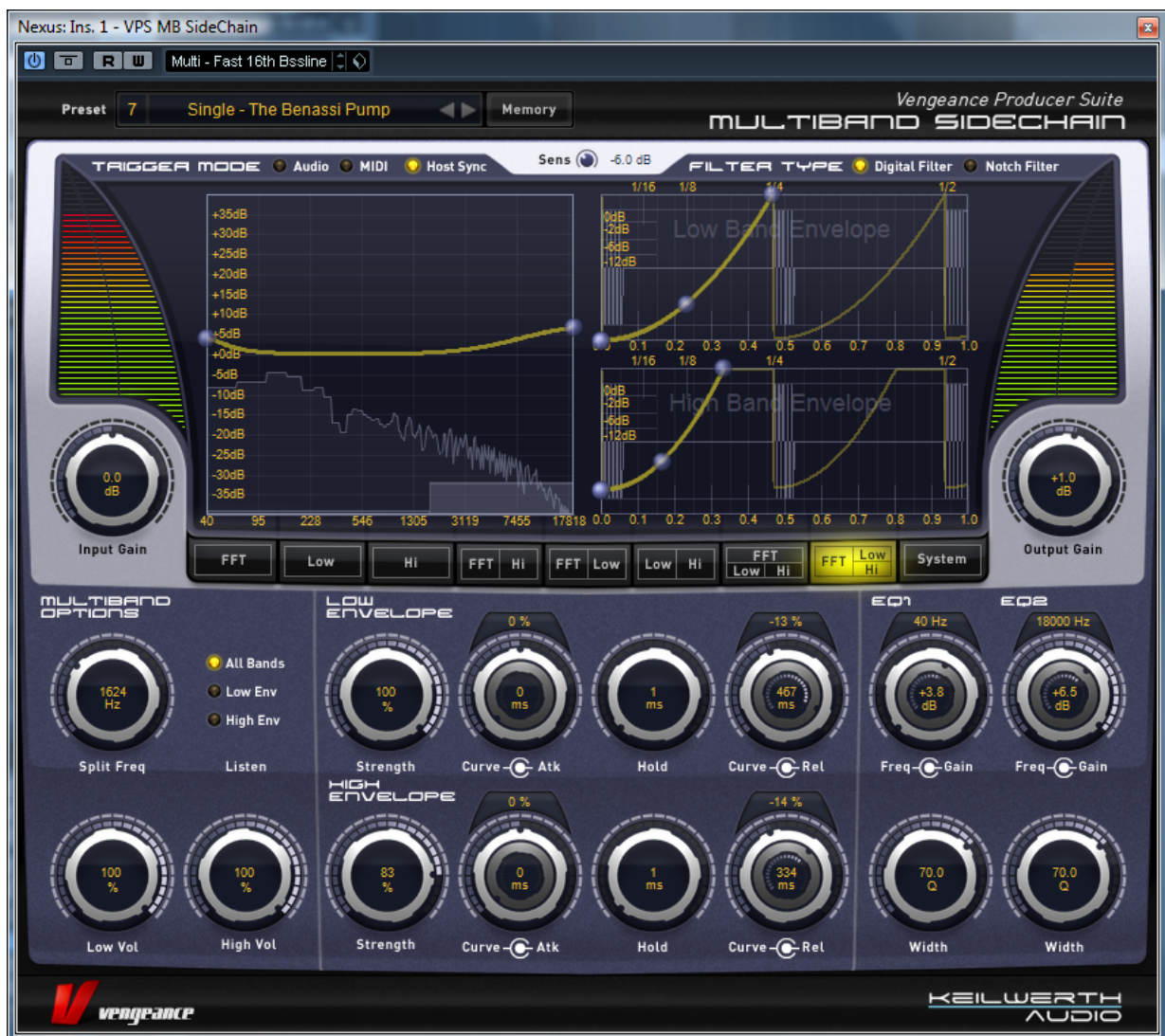
The VPS MBS window, full view
