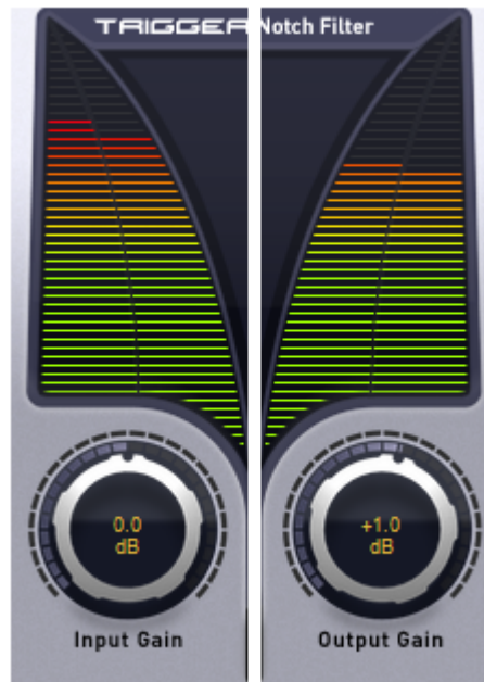
The VPS MBS level meters and gain controls
